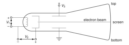
Which change in voltage results in the position of the spot on the screen moving towards the top?
